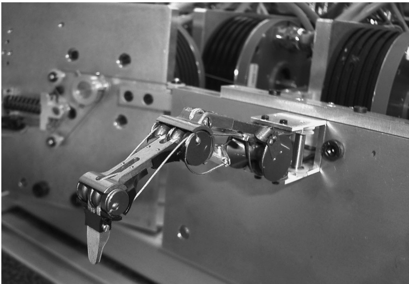
Figure 11. Realization of the first antagonistic finger of the DLR hand–arm system in a test bed. The drives and flexible elements of the test bed can be clearly seen in the background.
